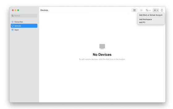
• Click on "Devices", use the "+" button to add a PC, then enter the computer name of the remote server you intend to connect to.
